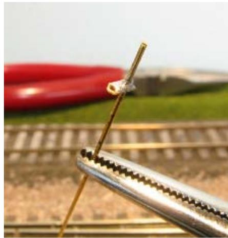
**Left:** Here is one of the vertical shafts, shown upside down, with the crank soldered in place. The dimension between the holes in the crank is very critical to achieve the 90-degree rotation. I made several attempts, before getting them right.
