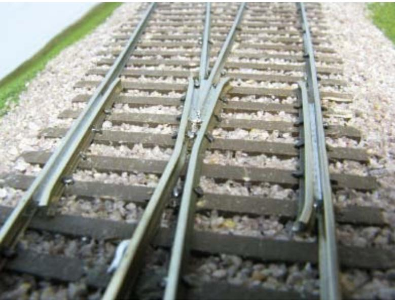
The turnout frogs are made by cutting and bending pieces of rail. The frog is then soldered, and the flange ways are opened up using a cut-off hack saw blade.
