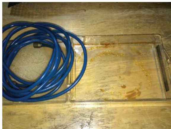
Air hose oozing oil in storage for 33 years.
