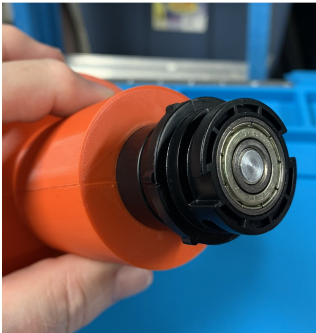
Split hub design with rotating spool holder.
