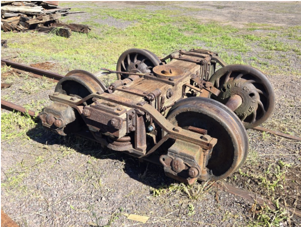
One of rock car #36's trucks. Note "Q M Co." and the date molded on the inside of the wheel.
