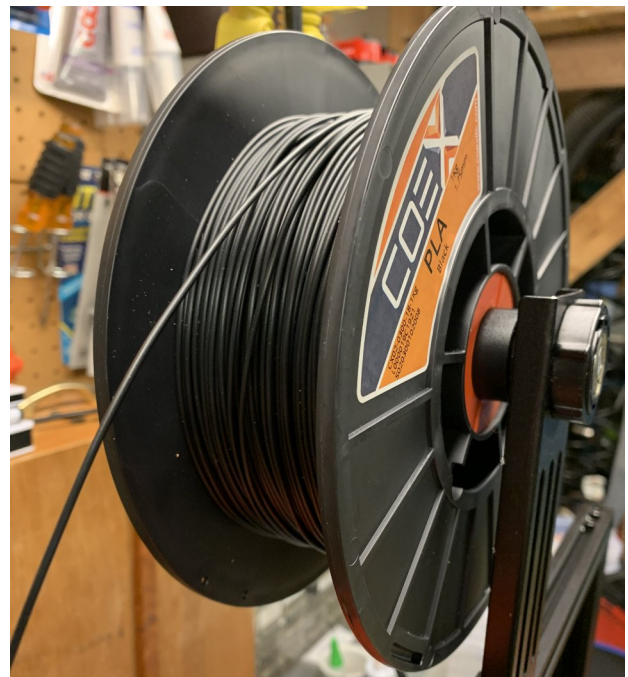
Filament spool does not rotate backwards with split spool hub.
