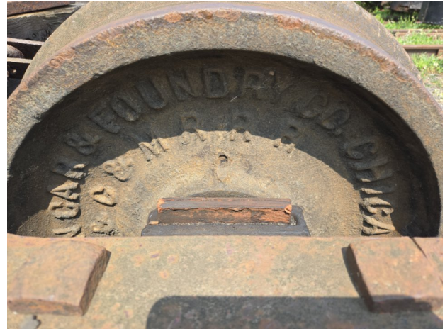
Wheel from rock car #36, showing "H&C&MRRR" and "American Car & Foundry Chicago" markings.
