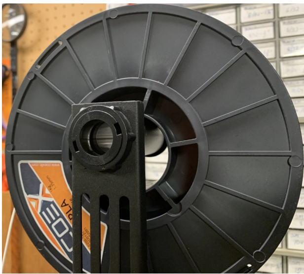
Filament spool sitting on a non-rotating spool holder.
