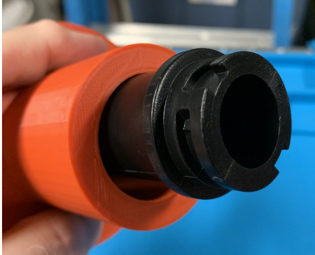
Spool hub slid onto non-rotating spool holder.
