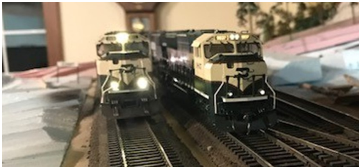
Figure 1: direct-install LEDs (left) vs factory light-piped (right).
