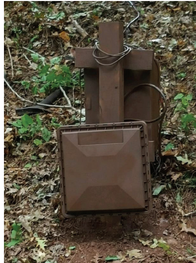
A close-up photo of an automatic equipment identification reader found in New Jersey.
