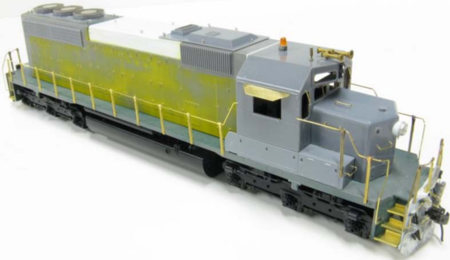
Above: This is a view of the shell before paint. The long hood received new fans and grilles from Cannon and Co.. New railings and brass etched steps were also added. Note the unique nose mounted bell, attached as on the prototype of this loco without a notch cut into the nose for flush mounting.
